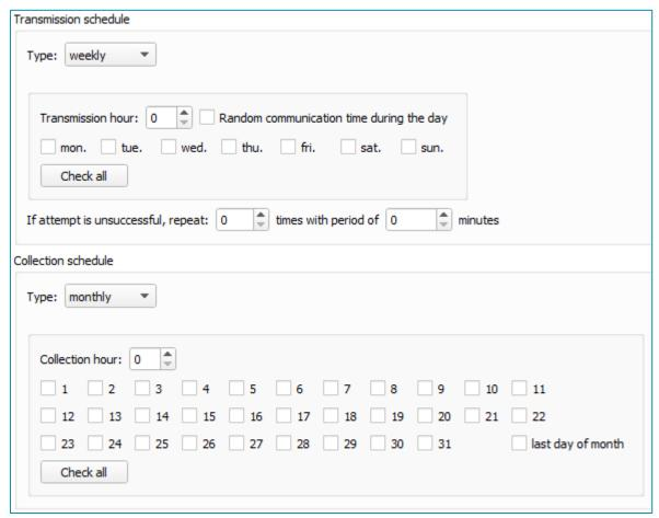
**Transmission schedule** – in this part the data transmission schedule is set. While weekly or monthly schedule is choosing you can use option "Random communication time during the day" or set the hour for transmitting data in the field "Transmission hour".
