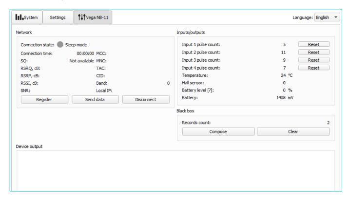
**Network** – displays the current parameters of the connection and allows to control it. Buttons in this block have logic like INIT button on the board.
