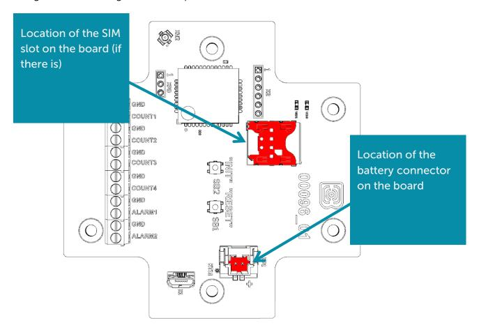
Vega NB-11 modem powered by the built-in battery which comes with. After battery connection the device loading and switch to the 'Sleep' mode until the communication session according with the schedule.
